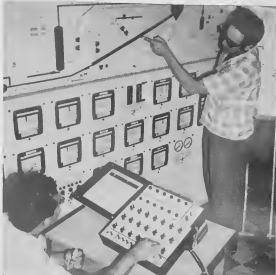
CARMODY TRAINING instructor F. Maduro at remote-control console directs B. Croes, a Process employee, on the operation of the ENTRENADOR CU e aparato Carmody. F. Maduro, na tablero di control remota ta dirigi B. Croes, un empleado di Process, com mester traha e planta di craqueo catalitico.
